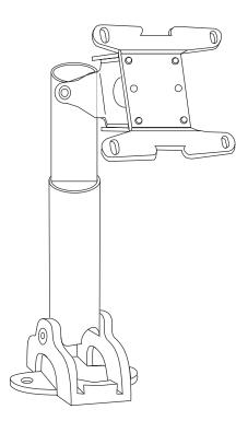
Typical Pedestal Type Mount with Swivel Bracket
